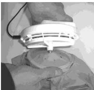
After checking whether the rubber ring is correctly attached, attach the flexible hood to the bottom of the main unit by attaching the press-stud.
